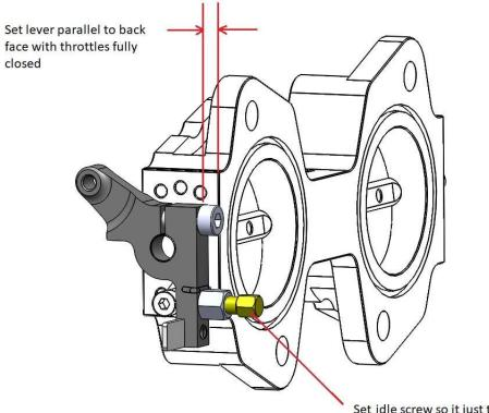
Set idle screw so it just touches the stop with throttles fully closed
