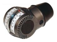
Press the synchronizer into each spacer. Adjust the balance coupling until the flow into each runner is exactly the same. Adjust the cable back down so the throttles are fully closed again.
