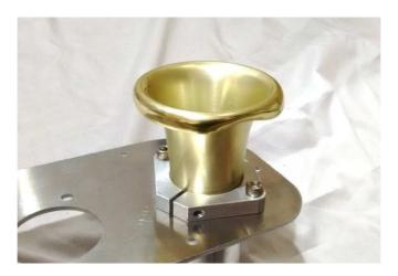
Assemble the two end trumpets and spaces to the backing plate with the clamping screws to the inside and the folded lip to the bottom of the last cylinder. Leave the bolts finger tight
