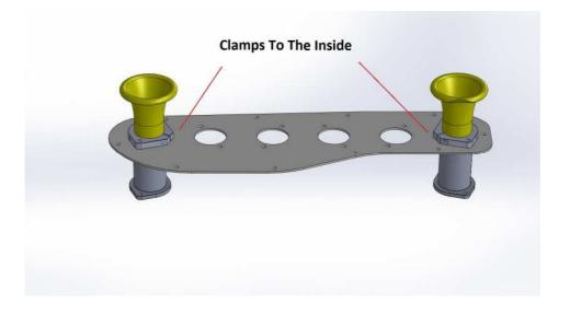
4) Check the fitment to the airbox and insert ALL the small fixing screws a few threads to ensure that all the screw holes line up, If they do not all insert then you may need to further fold the lip of the last trumpet, or you can slightly enlarge all the holes in the backing plate with a larger drill.
